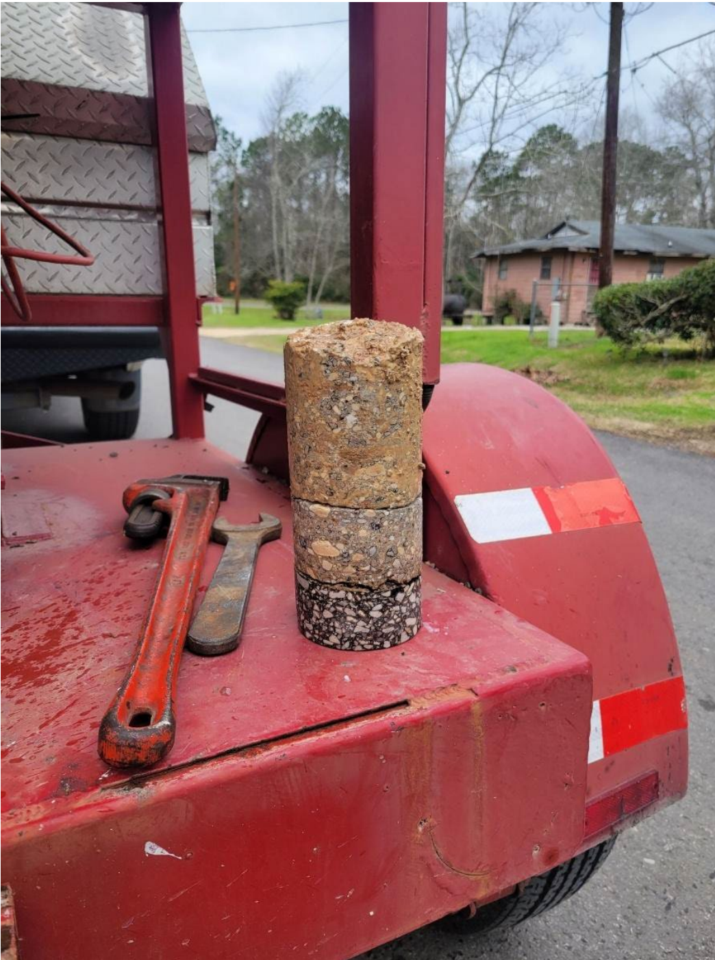
THICKNESS CHECK ON WESTWOOD. BASE (8") ASPHALT (2")
